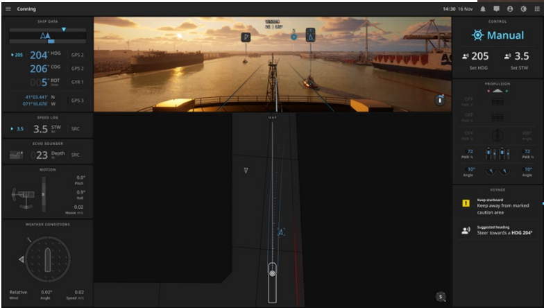
Bridge display with conning view with AR overlay on KMs camera cluster (KCC100 D) camera. (Source: OCIL)
