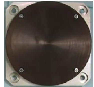
80mm long S-band patch antenna (Ref SSTL)
