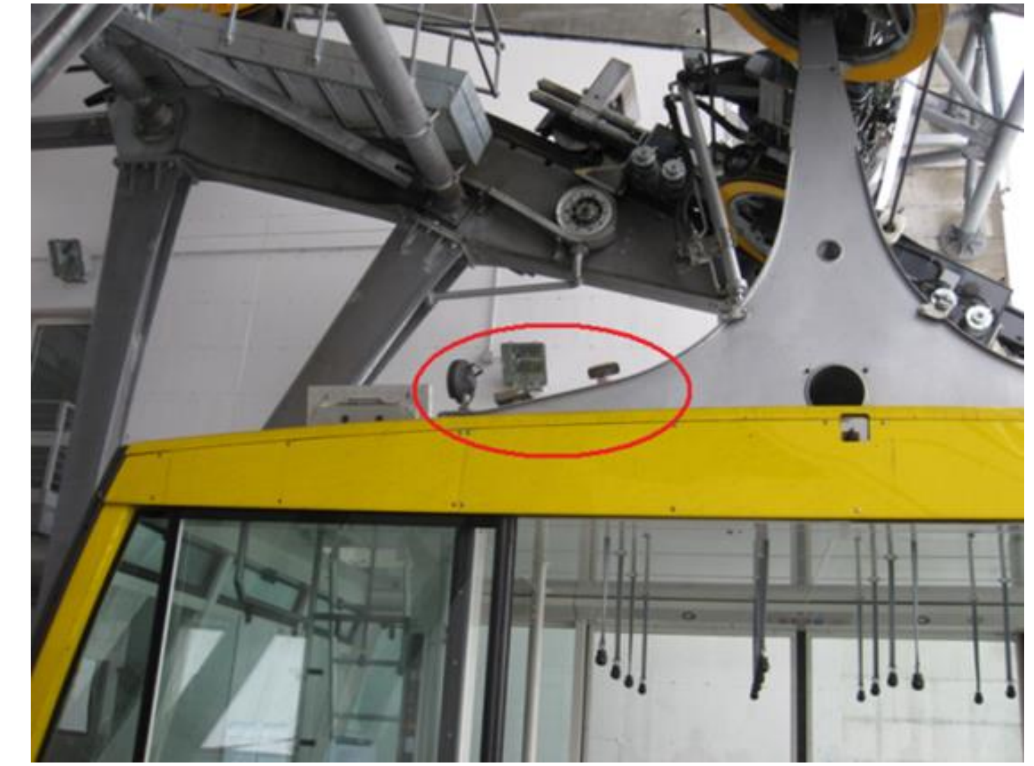
Fig. 1 Funifor - Ravascletto (UD) plant with the Topcon antennas on the roof of the cabin
