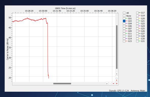
When the jamming starts, the signal is completely lost
