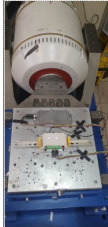
Photo of the Exciter connected to a test bed with the Industrial Gateway mounted on a DIN rail in its X and Y- axis test configuration
