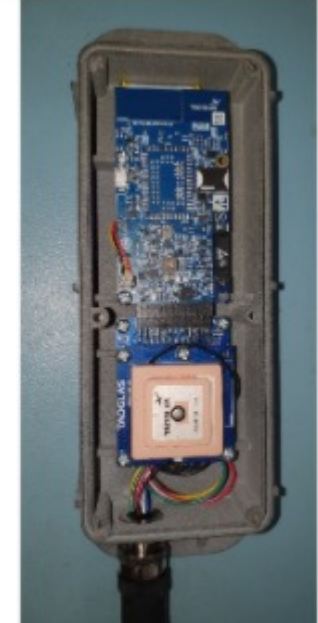
Image of the Edge Rugged with communications cable attached to the unit. The top cover is off to show the internal connections.
