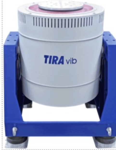
Image of the Electrodynamic exciter TIRA vib used for this testing
