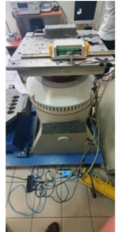
Photo of the Exciter connected to a test bed with the Industrial Gateway mounted on a DIN rail in its Z-Axis test configuration
