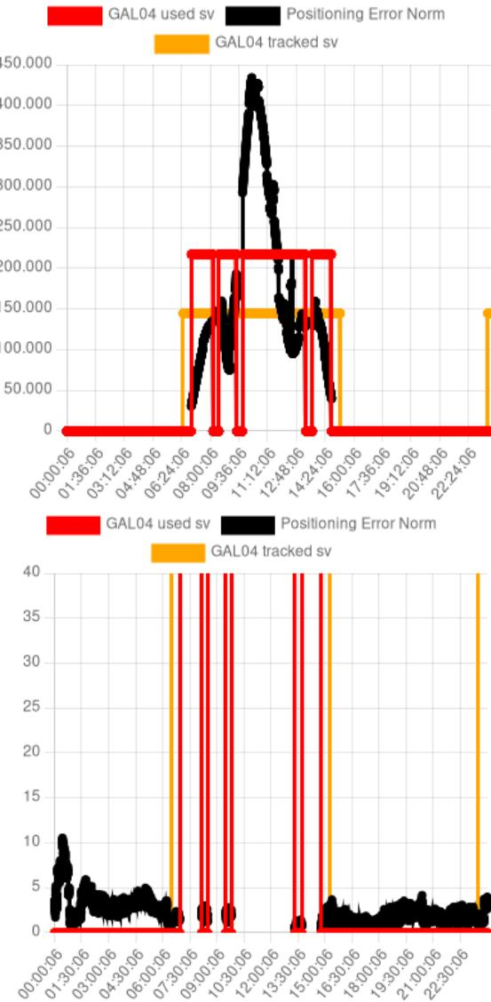
The trend of the positioning error norm has a very high value only in those epochs where the E04 satellite has been used. In the left side plot there is the case of 25 November and in the right the case of 26 November.
