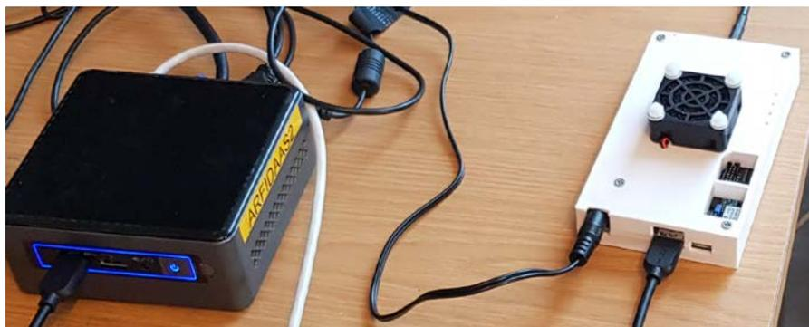
Figure 2: ARFIDAAS NUC PC on left connected to enclosed Front-end on right.
