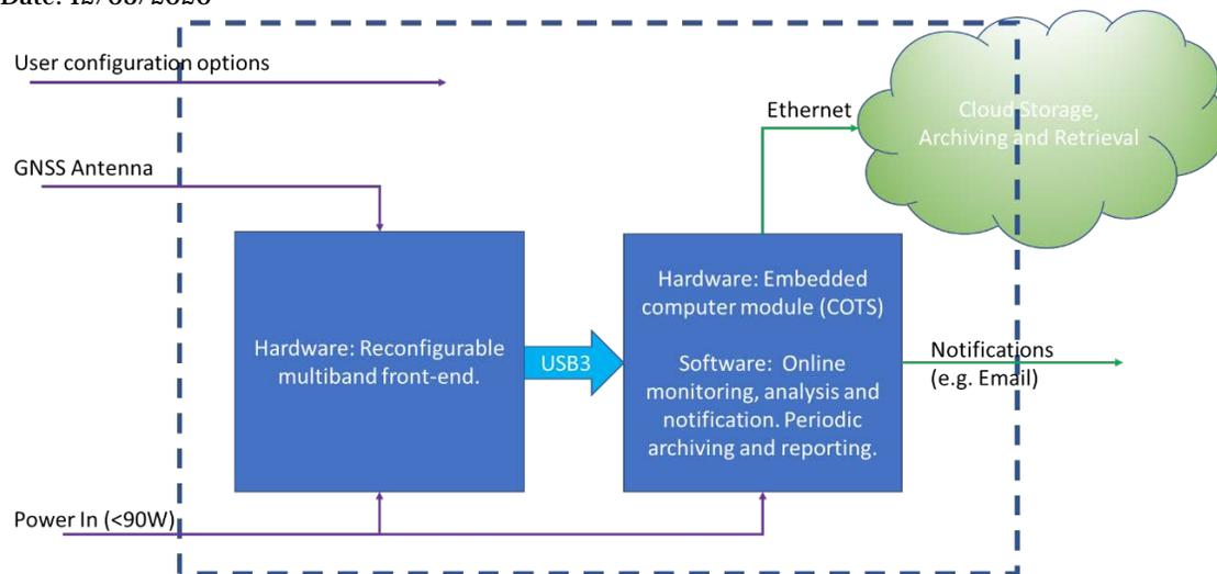
Figure 1: ARFIDAAS system block diagram
