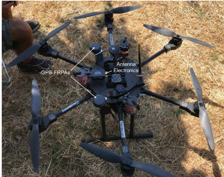
Figure 2 - UAS with two FRPAs and inline anti-jam antenna electronics
