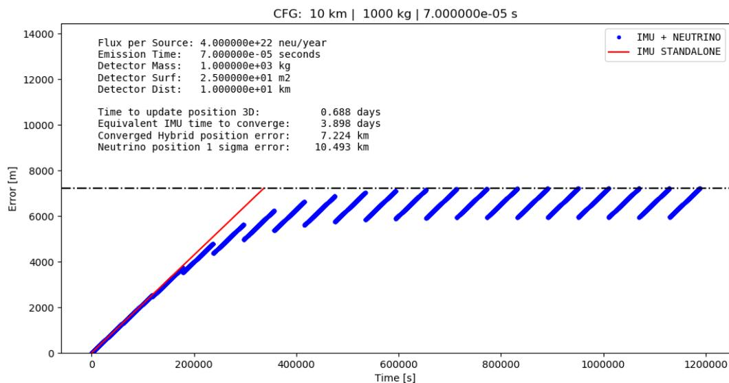
**Figure 1-3 Hybrid and IMU standalone solution for an accuracy requirement of 10 km and 1000 kg of detector mass**
