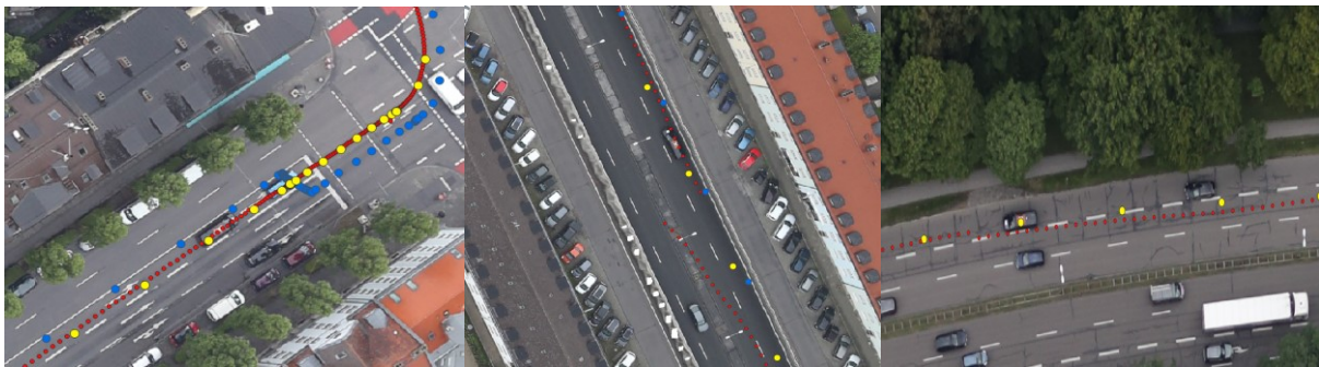
Figure 1 - Examples of performance deviations of both the automotive and high grade GNSS sensors. As seen, even for the positions of the high-grade sensor with RTK corrections (red), deviations of varying degrees occur in urban environments compared to the automotive receiver (blue) and the positions derived from aerial imagery (yellow)
