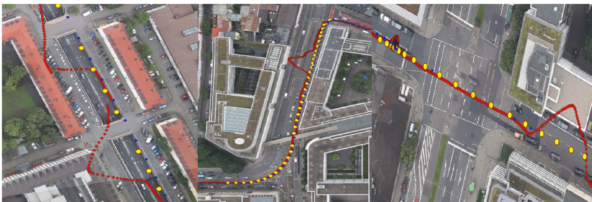
Figure 2 - Examples of performance deviations of both automotive and high grade GNSS receivers. As seen even for the positions of the high-grade receiver without RTK corrections (red), deviations of varying degrees occur in urban environments compared to the automotive receiver (blue) and the positions derived from aerial imagery (yellow).
